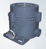
CPS/EMH.. series enclosures offers Ex dB IIC mode of protection and is equipped with window made of tempered glass for electrical equipment which requires a direct reading from the outside.
